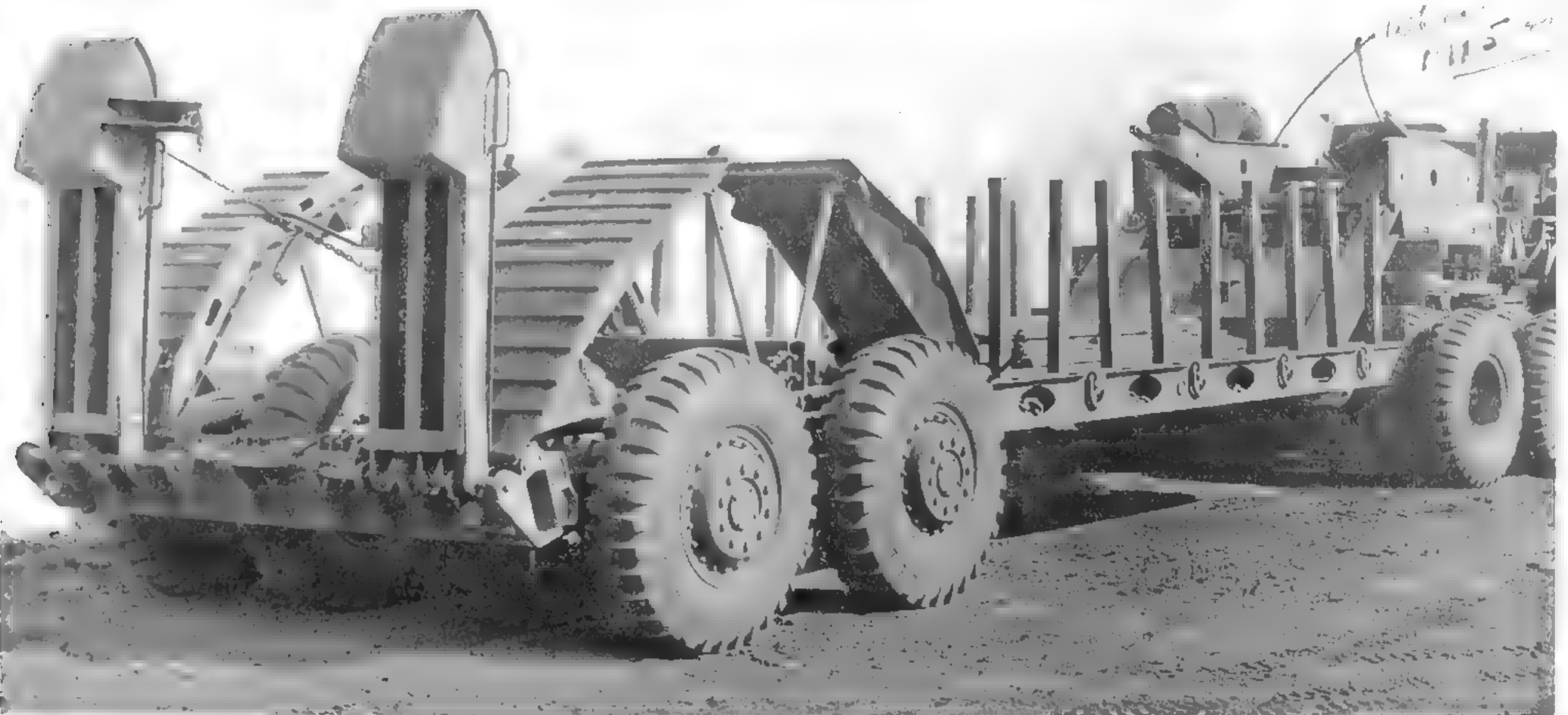
The hinged rear wheel covers of the M15A1 are clearly visible here. This is the pilot model, and ironically still carries the removable covers of the M15, as pointed out by the notation of the wartime editor. (U.S. Army photo)
